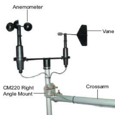
The 03001 is secured to one end of the CM206 crossarm with the CM220 Right Angle Bracket.
