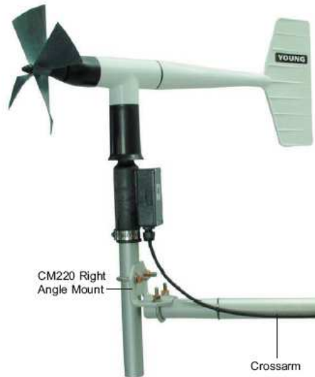
The 05305 Wind Monitor-AQ provides high accuracy measurements, typically for air quality applications.
