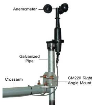
When purchased separately, the Wind Sentry Anemometer is supplied with a galvanized 10" x \frac{3}{4} " diameter threaded pipe, which mounts to a crossarm via a CM220 Mount or NU-RAIL fitting. Alternately it can mount to an stainless-steel tripod via the CM216.
