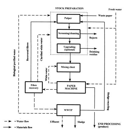
Figure 5.6: Basic flow chart of the recovered paper processing paper and board production [Dutch Note on BAT, 1996]; WWTP = Wastewater Treatment Plant
