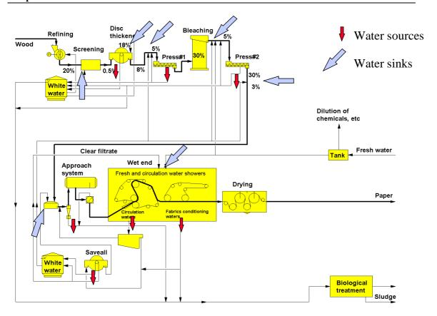
Figure 4.8: Main water sources and sinks in an integrated mechanical pulp and paper mill [Edelmann, 1997]
