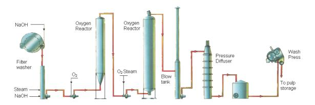
Figure 2.10: Two-stage oxygen delignification
