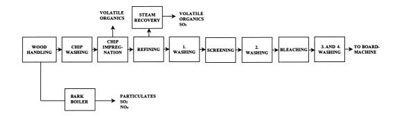
Figure 4.7: Emissions to the atmosphere from CTMP mills
