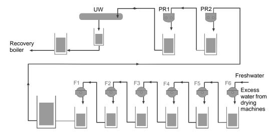
Figure 2.11: Possible water system in closed up bleach plants
