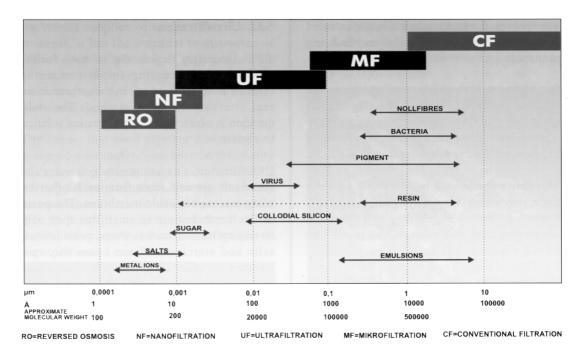
Figure 6.11: Filtration ranges of different filtration technologies
