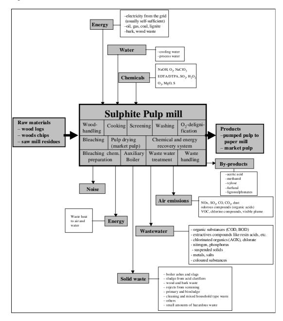
Figure 3.3: <u>Mass stream overview of a sulphite pulp mill.</u>
