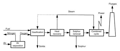
Figure 2.14: Integrated gasification with combined cycle (IGCC).
