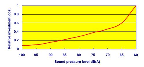
Figure 6.24: Relative costs of external sound attenuation [according to Valmet].
