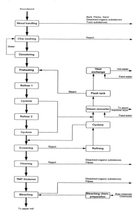
Figure 4.3: Schematic of the TMP process and emissions [SEPA Report 4713-2, 1997]
