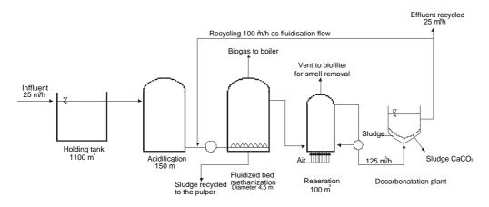
Figure 5.12: Example for an industrial in-line treatment in a zero effluent mill manufacturing corrugated medium [Niovelon, 1997]
