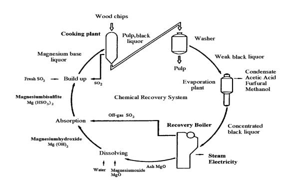
Figure 3.2: Recovery cycles for a sulphite mill
