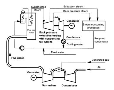
Figure 2.15: Combined cycle for power production by means of gas turbine and steam turbine with condensing tail.
