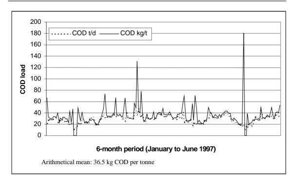
Figure IV.4: Daily average COD emissions to water from a kraft pulp mill over 5-month period
