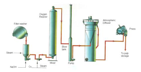
Figure 2.9: One stage oxygen delignification
