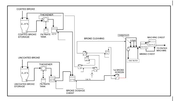
Figure 6.4: Possible lay out of a broke system of a paper mill manufacturing coated paper. Uncoated and coated broke are stored in separate tanks.
