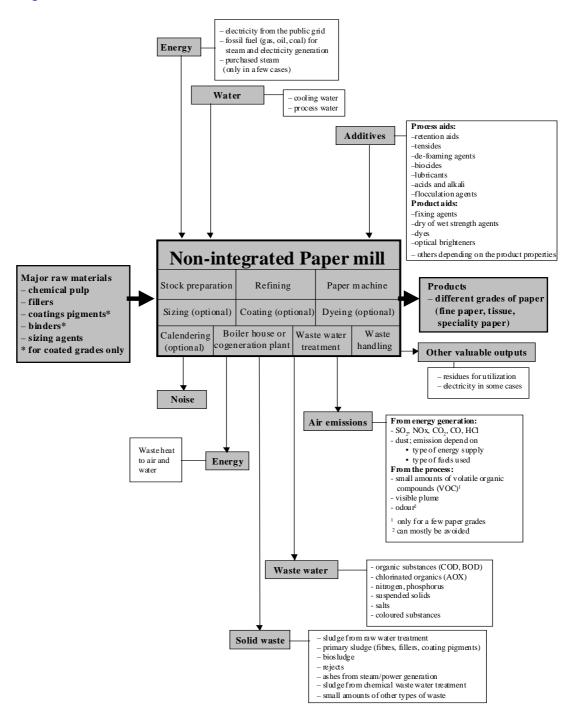
Figure 6.6: Mass stream overview of a paper mill.
