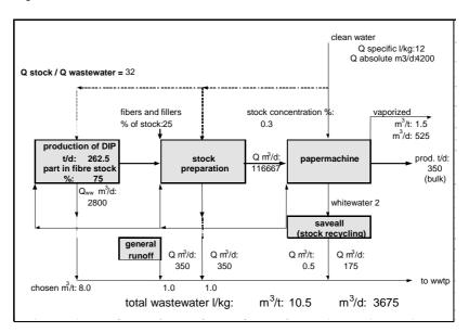
Figure 5.8: Example of an optimised stock-water-system for an integrated production of de-inked pulp
