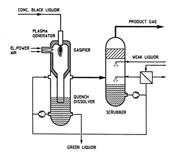
Figure 2.13: The Chemrec process with a gasifier and a quench dissolver for green liquor production and with a weak liquor gas scrubber for hydrogen sulphide absorption
