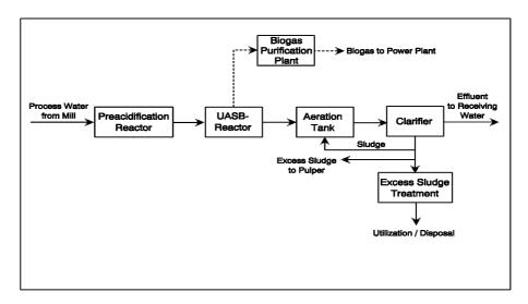
Figure 5.14: Simplified scheme of a combined anaerobic/aerobic wastewater treatment plant [IFP, 1998]
