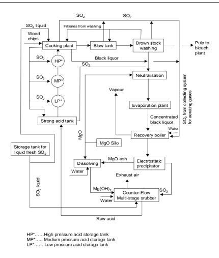
Figure 3.7: SO<sub>2</sub> - circuit in a sulphite pulp mill
