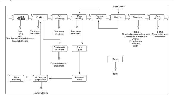
Figure 2.5: Emissions to water from a kraft pulp mill
