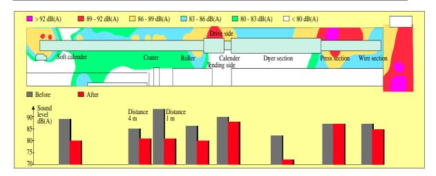
Figure 6.10: Machine room noise levels before and after the rebuild in different sections of a paperboard mill.
