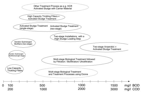
Figure 6.14: Main processes for external treatment of paper mill wastewater and the ranges of suitable application.
