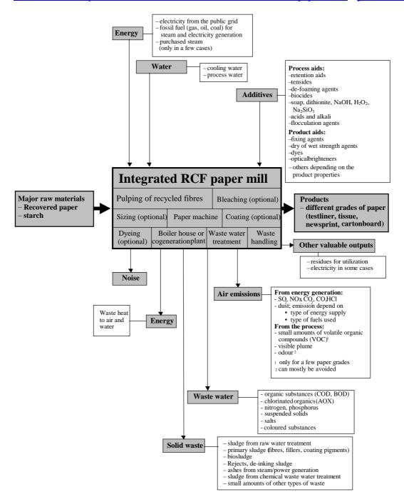
Figure 5.5: Mass stream overview of an integrated recovered paper processing mill.
