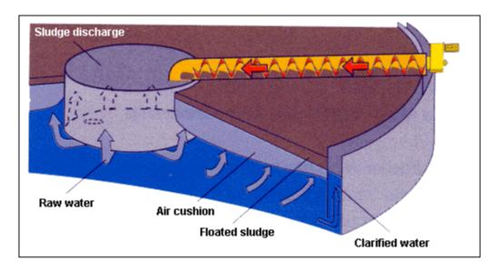
Figure 5.16: Operating principle of a dissolved air flotation (DAF) [M.Schwarz, 1995]
