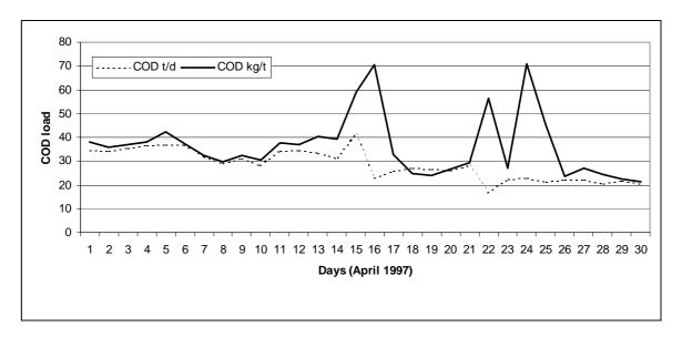
Figure IV.3: Daily average COD emissions to water from a kraft pulp mill over 30-day period
