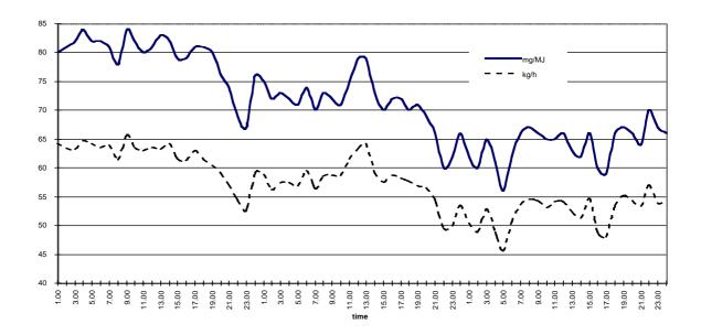
Figure IV.1: Continuous monitoring data of NOx emissions from a kraft recovery boiler over a 3 days period.
