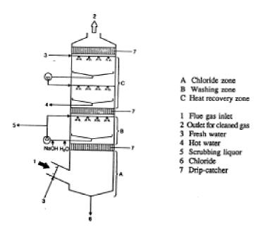
Figure 2.12: Flue gas scrubber for recovery boilers [SEPA-Report 4008, 1992]
