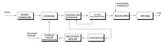
Figure 3.1: Main unit processes of manufacturing of magnesium sulphite pulp [CEPI, 1997b]
