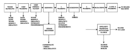
Figure 4.6: Emissions to water from a CTMP mill
