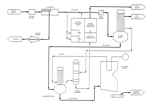
Figure 4.10: Zero liquid effluent process concept [Ward, 1993]
