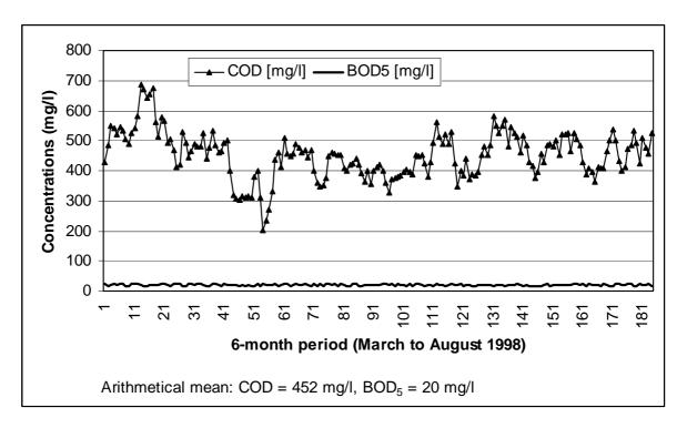
Figure IV.6: Daily average emissions to water from an integrated sulphite pulp and paper mill over a 6-month period
