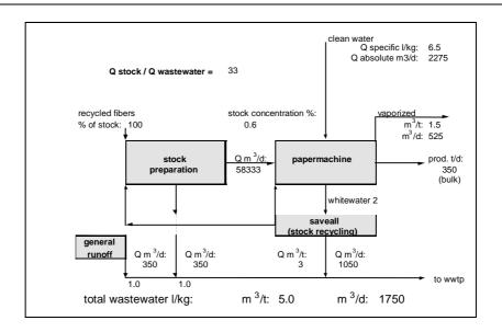
Figure 5.7: Example of water circuits for an integrated RCF mill for corrugated medium without de-inking (100% recovered paper)
