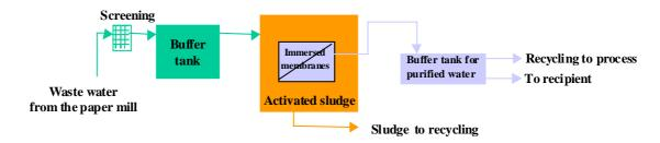
Figure 5.19: Membrane bioreactor using immersed membranes in an activated sludge reactor
