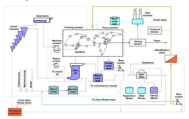
Figure 6.12: Possible simplified lay out for a paper mill using ultrafiltration for white water purification.
