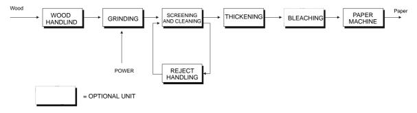
Figure 4.2: Groundwood pulping process
