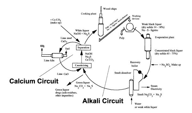
Figure 2.3 Recovery cycles of chemicals for a kraft mill
