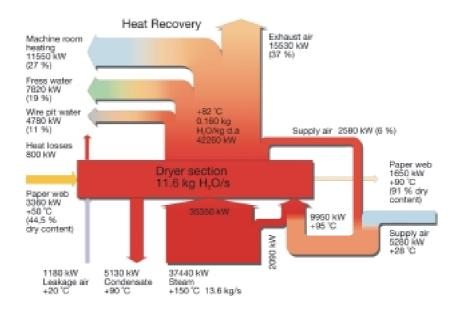
Figure 6.21: Sankey diagram for a newsprint machine (980 t/d).
