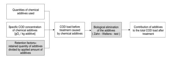
Figure 6.15: Pragmatic approach for assessment of the amount of heavily biodegradable additives to be expected in effluents from paper mills after treatment [IFP, 1997]
