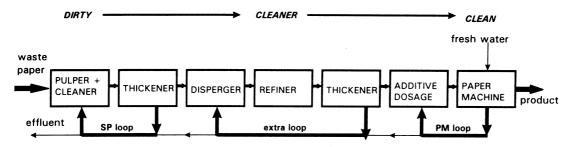
Figure 5.11: Lay out of water loops in a paper mill with separation of water loops and countercurrent flows
