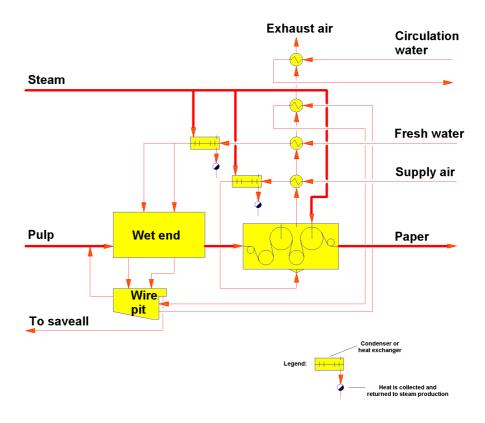
Figure 6.2: Paper machine heat recovery system
