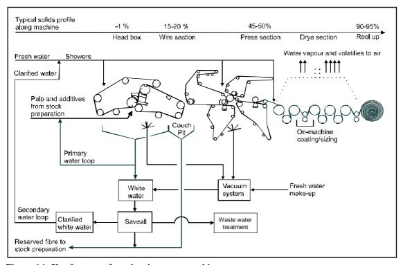
Figure 6.1: Key features of a twin wire paper machine
