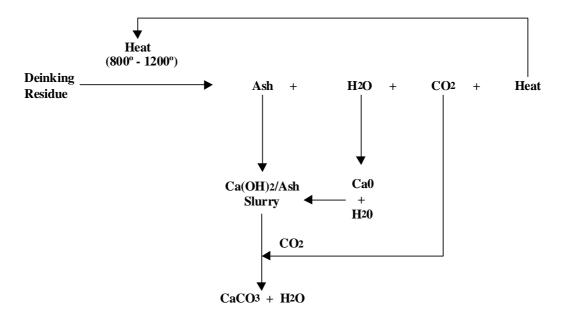
Figure 5.20: The main principles of the RMF PCC process Reproduced from "Recycling of Mineral Fillers from the Residue of a Paper Deinking Plant", Sohara et. al., U.S. 5,759,258, 1998
