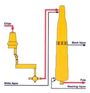
Figure 2.2: Continuous digester
