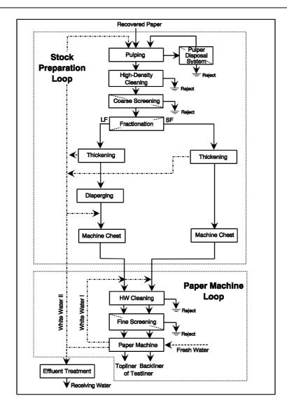
Figure 5.1: Flowsheet of an example for a stock preparation plant concept for processing recovered paper for case making material (2-ply testliner)
