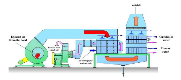
Figure 6.20: Example for a heat recovery tower.
