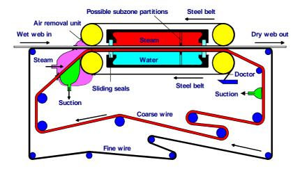
Figure 6.26: Schematic of the Condebelt<sup>®</sup> drying process (high Z-pressure type)
