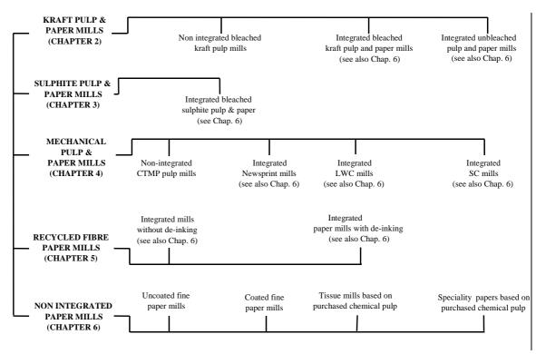
Figure 1.7: Classification of pulp and paper mills proposed by this document including cross-references to the relevant chapters for those mills.
