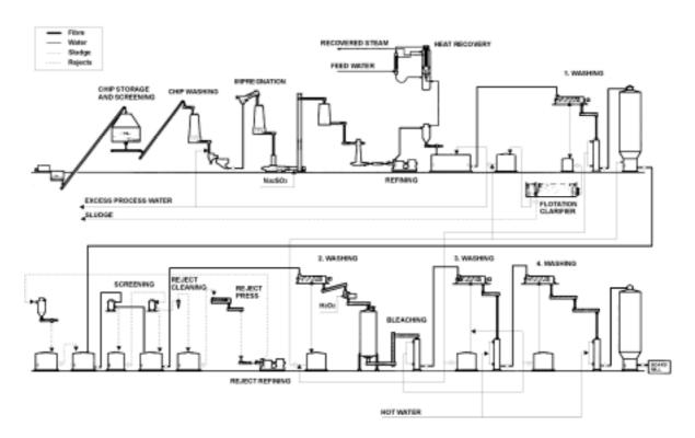
Figure 4.4: Schematic of the CTMP process [By courtesy of a Finnish mill, 1998]
