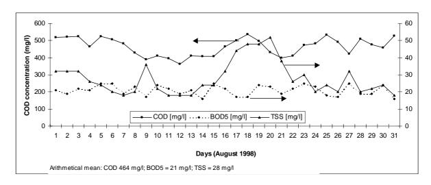
Figure IV.5: Daily average emissions to water from an integrated sulphite pulp and paper mill over a one-month period
