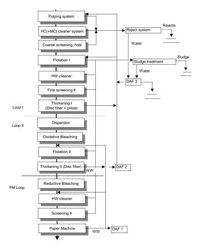
Figure 5.3: Example for an overall plant concept for (improved) newsprint There are also other approaches to newsprint line process configurations
