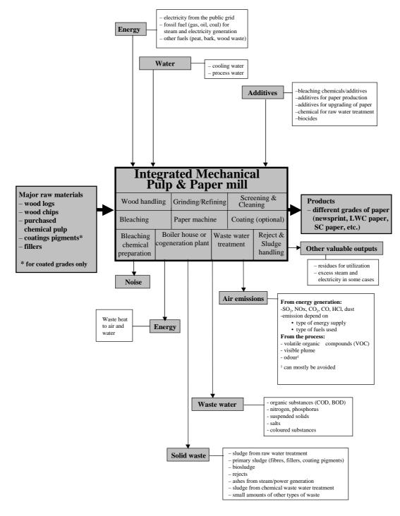
Figure 4.5: Mass stream overview of an integrated mechanical pulp and paper mill. The presence of some of the substances depend mainly on the paper grade and paper properties to be achieved and the type of energy supply
