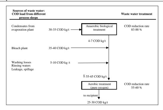
Figure 3.5: Wastewater load from sulphite pulping and treatment systems including reduction efficiency. Example of organic loads before and after treatment from a German sulphite pulp mill.
