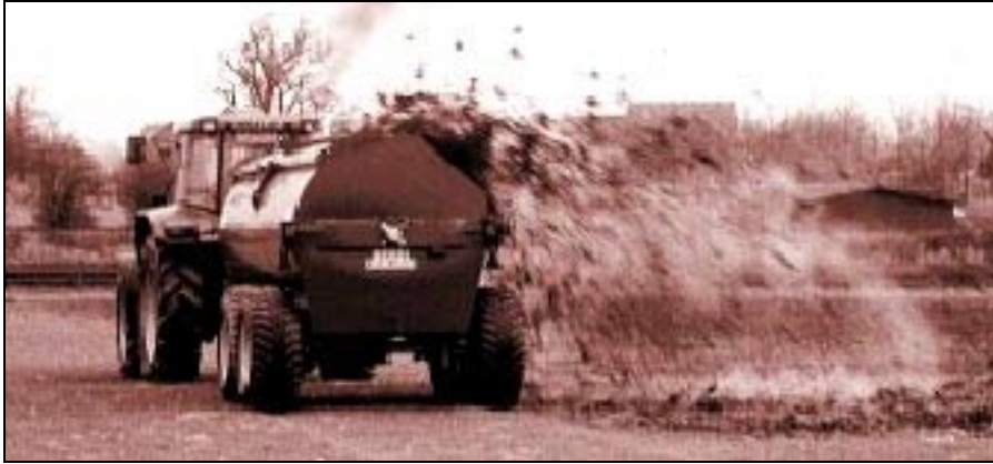
Figure 2.44: Example of a rotaspreader [51, MAFF, 1999]
