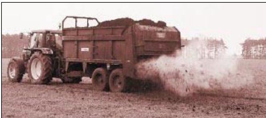
Figure 2.45: Example of a rear discharge spreader [51, MAFF, 1999]
