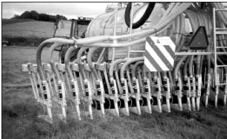
Figure 2.41: Example of a trailing shoe spreader [51, MAFF, 1999]
