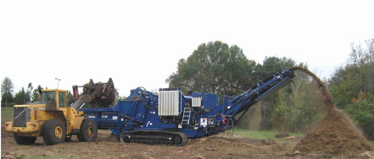
Photograph 4.4: Raw Materials Shredding – Using a High Speed Shredder
