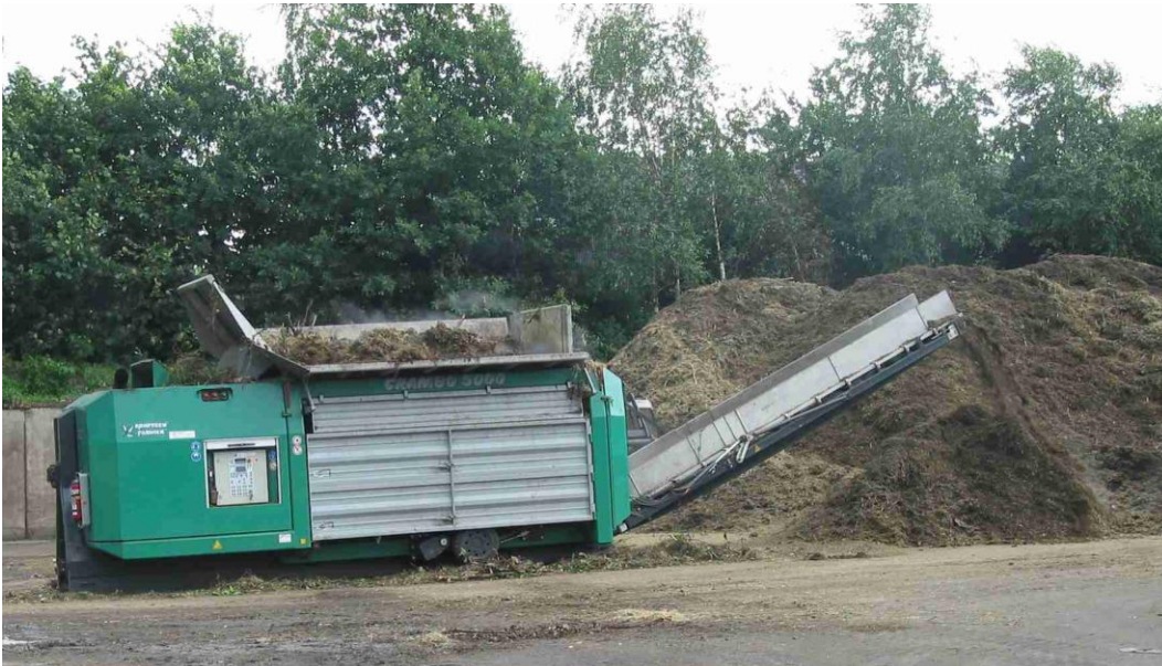
Photograph 4.3: Raw Materials Shredding – Using a Low Speed Shredder
