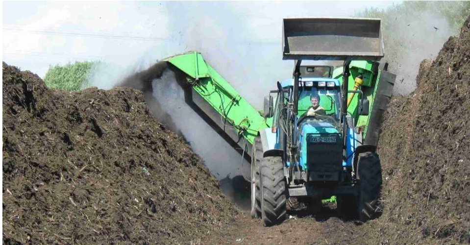
Photograph 4.6: Windrow being turned by a side turner
