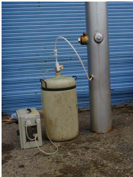
Figure 3.3: Odour sampling apparatus
