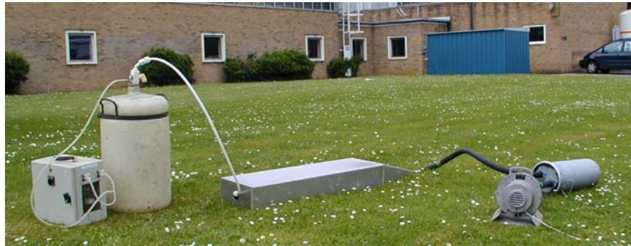
Figure 3.11: Demonstration of a sampling train using a sampling hood
